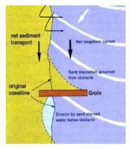
As sand accumulates on the updrift side of the groin, the beach at that location becomes wider. However, this is often accompanied by accelerated erosion of the downdrift beach, which receives little or no sand via longshore transport. It is important to realize that groins do not add any new sand to the beach, but merely retain some of the existing sand on the updrift side of the groin.
