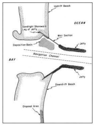
because seaward sediment transport from the beach along the outside of the jetty is minimized (Seabergh and Lane 1977).
