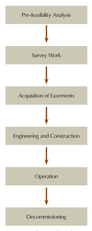
Figure 7. Steps of transmission line development.
