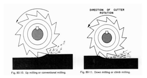
iv. <u>MILLING MACHINE SPEEDS AND FEEDS</u> Cutter speeds (fpm)(spindle speed) vary according to the diameter of the cutter, cutter material, the recommended cutting speed for the specific material, and the cutting fluid used. Feed rates vary by the type of cutter, number of cutter teeth, rigidity of the machine and setup, and rough or finish cut.
