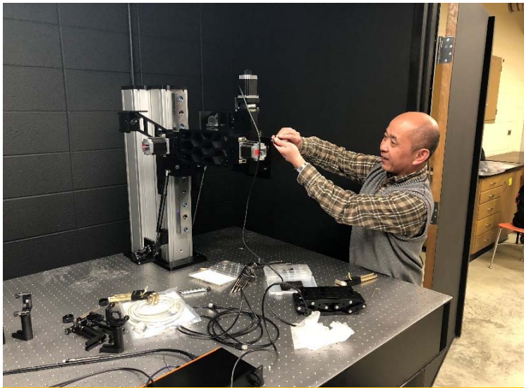
Core director, Dr. Zhang, is installing a PMT, which is a critical part of the two-photon microscope.
