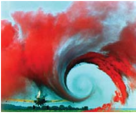
Fig 1. Illustration of an airplane vortex (from Wikimedia Commons). Corresponding unsteady, separated flow regimes are found with regard to many highly essential problems, e.g. regarding the assessment of the performance of wind farms and effectiveness of aircraft designs.
