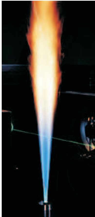
Figure 5.2: Photograph of flame III. The area covered is approximately 72 (height) \times 25 (width) cm. (Courtesy of R.S. Barlow, Sandia National Laboratories).
